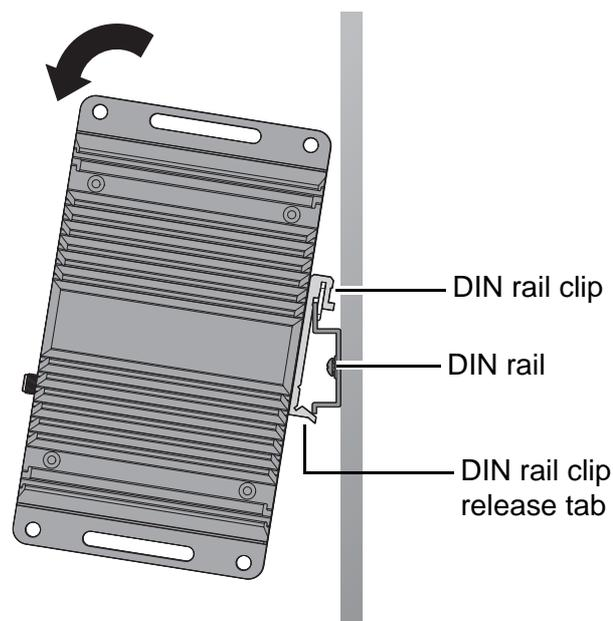
**Figure 2.5 Installing the DIN-Rail Mounting Kit**
