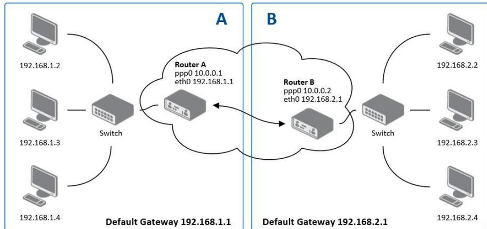
**Figure 3.28 Topology of GRE Tunnel Configuration Example**
