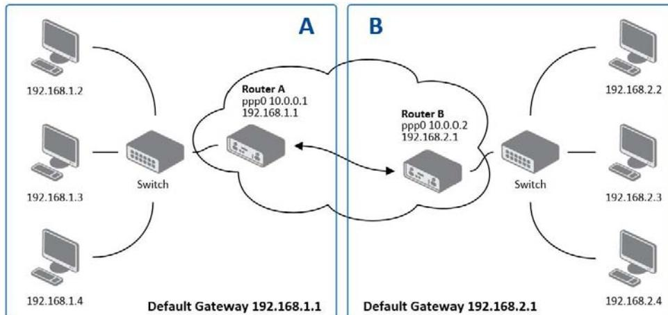
**Figure 3.32 Topology of PPTP Tunnel Configuration Example**
