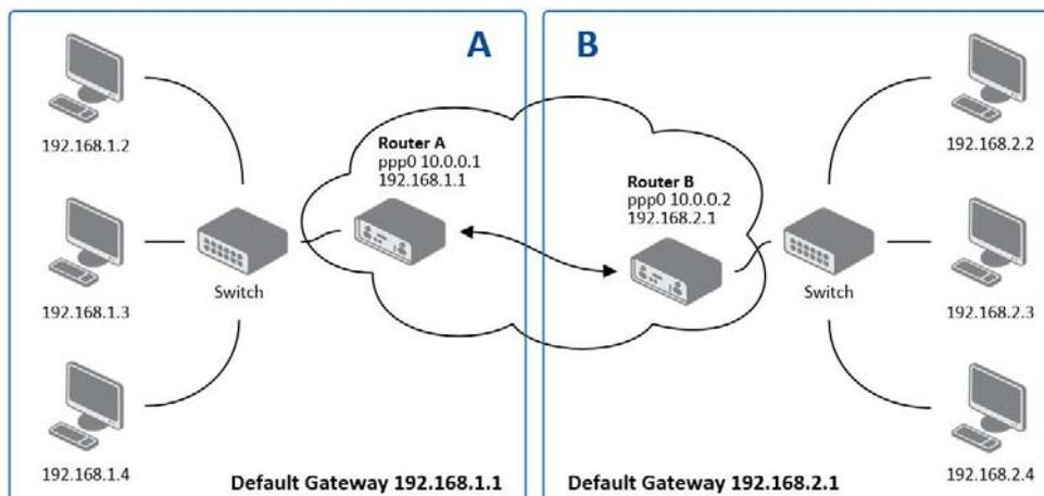
**Figure 3.30 Topology of L2TP Tunnel Configuration Example**
