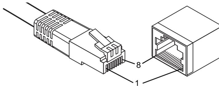
Figure 2.8 Ethernet Plug & Connector Pin Position
