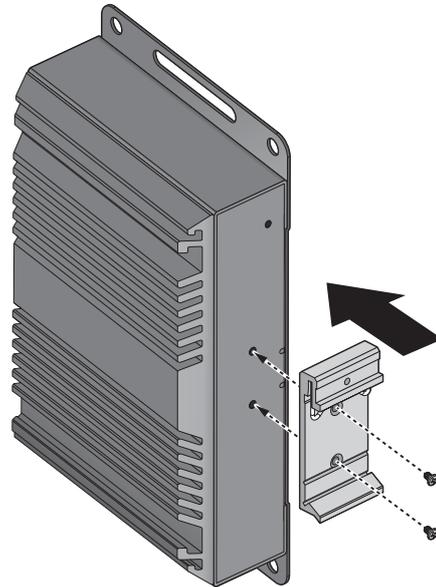
**Figure 2.4 Wall Mount Installation**
