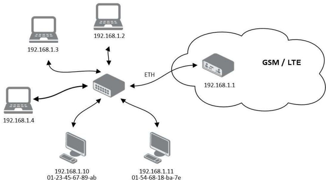
**Figure 3.14 IPv4 Dynamic and Static DHCP Network Topology**
